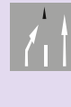
Lane reduction ahead. Warns that a lane discontinues ahead, and traffic from the side indicated will merge into the continuing lane.
