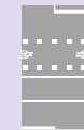
Cycle crossing. Cyclists cross the road at the place indicated by the broken lines.
