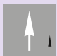
Direction of travel indicators. Indicate the direction in which vehicles may travel.
