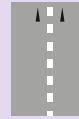
Lane line. Short, thin lines to separate lanes of traffic moving in the same direction; the gaps may be longer or shorter.
