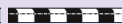
Kerbing marking. To indicate the presence of a raised sidewalk or island kerbing.
