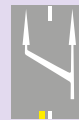
End of exclusive use lane. Warns that the exclusive use lane ends here.
