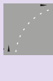
Guide lines. These broken lines indicate where a vehicle should position when turning, or where there is a shift in the road alignment, or where pedestrians should cross.
