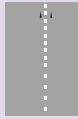
Continuity line. The roadway to the left of the thick marking discontinues straight ahead; the gaps become progressively shorter as the line continues.
