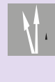
Furcation arrows. There is an increase in the number of lanes ahead, in the direction/s indicated by the arrows.
